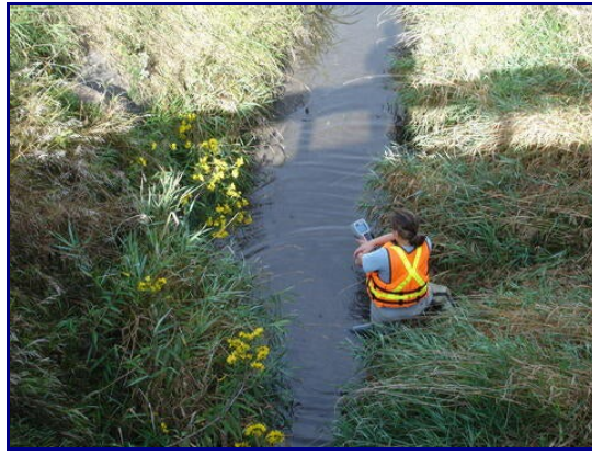
Scientist measuring baseflow levels of a stream. (US Geological Survey)
